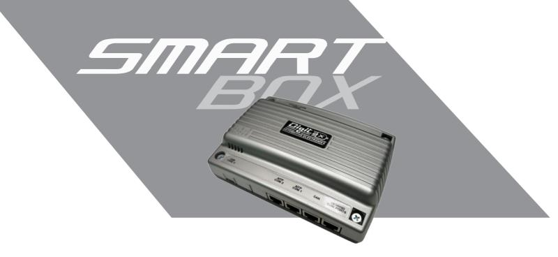
The Smart Box comes with a simple and ready-to-use Android SDK that allows you to easily integrate often complex interfaces like CAN bus and Inputs/Outputs with your Android Apps.
