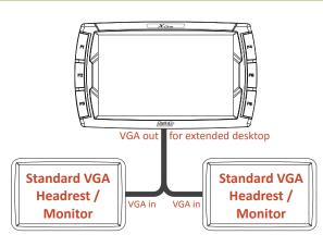
VGA Output compatible with market headrest monitor for passengers information media (PIM) with independent content from driver mobile data terminal
