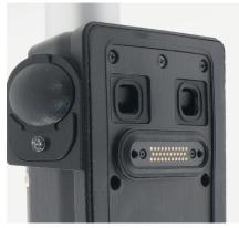
The **Pole Docking** is designed to provide **IP65**-rated protection, ensuring the waterproofing not only of the main unit but also of its connector. This is achieved through the use of a special **Pogo Pin**-type connector, which remains fully shielded from accidental infiltration, effectively **eliminating any risk of water ingress into the cable compartment.**
